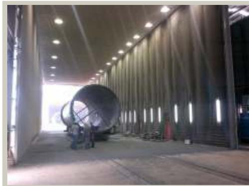
The blasting of wind towers requires high quality surface preparation and high production rates. Our wind tower blastrooms are designed and engineered to meet both of these requirements.
